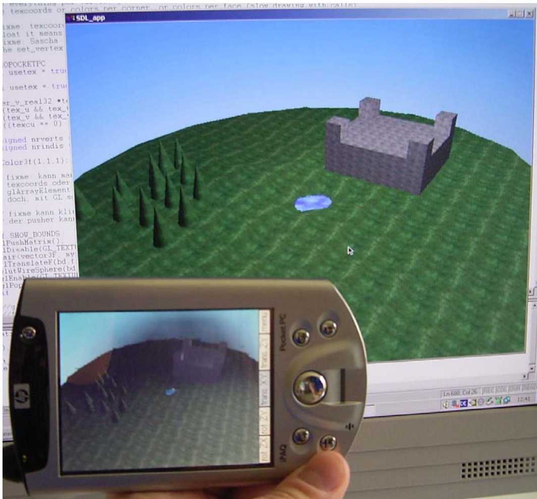
Figure 4: A textured verse scene downloaded from the Verse server and rendered on a desktop Verse viewer and at a PDA using the slim rendering client.
